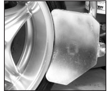
Extra caution is required when using a bead loosening blade.
