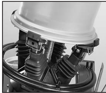
This “tulip” clamping system provides “soft grip” internal and external clamping.
