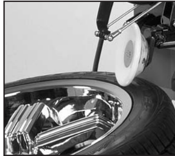
Bead rollers loosen the bead with minimal stress on the tire.
