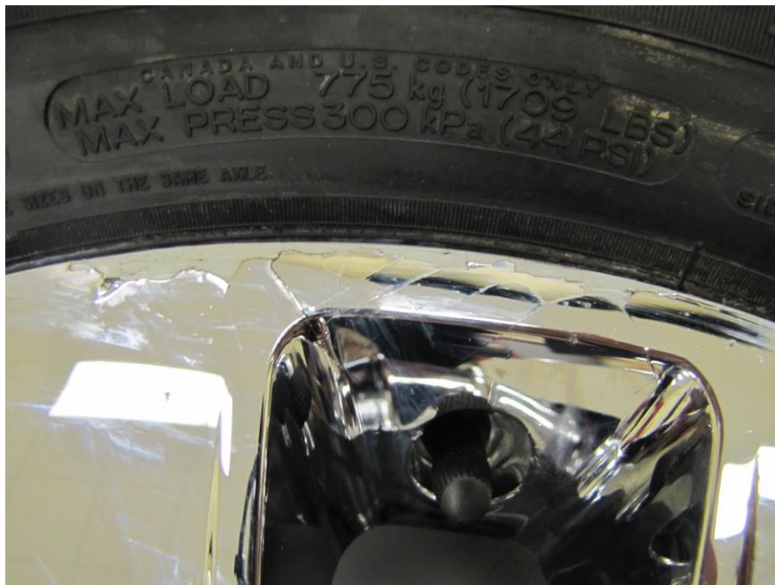
Damage caused by improper procedures
